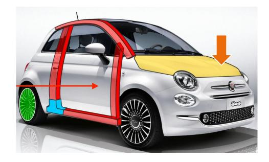
Cold reforming of external non-structural elements
