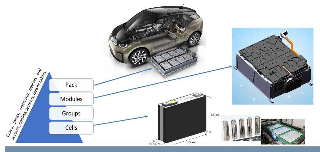
Substantial **differences in the design** of battery modules of different car manufacturers and availability of different types of joints within the same battery make the disassembly phase complex and challenging.
